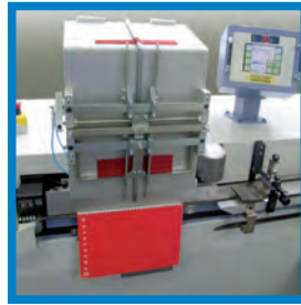
Touch screen and hanger feeder.
