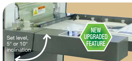
The new inclined feed table can be set level, or at 5° or 10° to aid semi-automatic feeding, which helps to increase productivity
