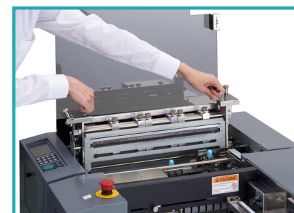
DC-516 Pro comes with one cutting module, one slitting module and one creasing module
