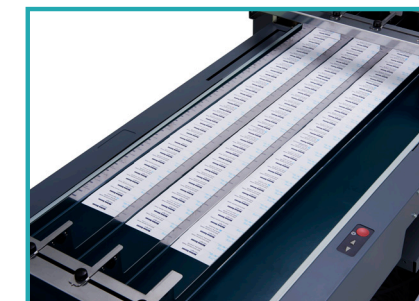
Long Conveyor handles stacking of high volume jobs
