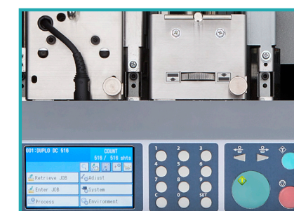
A color and user-friendly control panel stores up to 250 jobs for quick changeover
