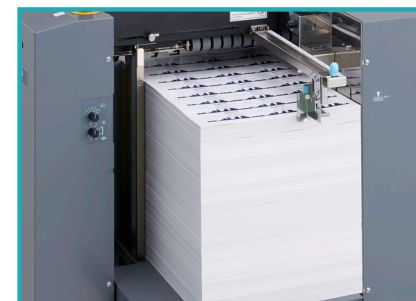
High pile feeder with 8-belt air suction feed system
