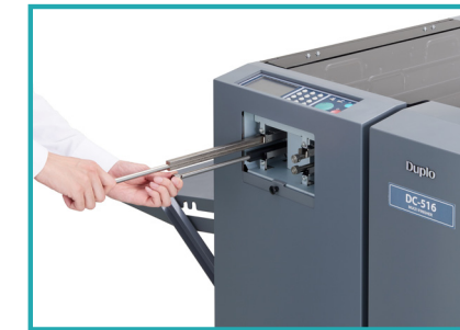
New creasing module includes a dual creasing tool with the capability to perform positive or negative patterns
