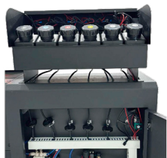
White ink stirring system, to avoid white ink clogging at printheads, ink shortage alarm system.
