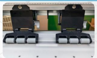
According to the printing film, the pressure of the pinch roller can be adjusted to ensure smooth paper feeding and high printing accuracy when printing.
