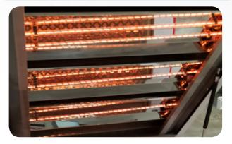
The upper and lower rows of infrared heating lamps and the closed oven make the temperature more uniform and help to quickly cure the powder.
