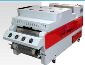
The integrated smoke purifier on the side can automatically process the smoke and discharge it.
