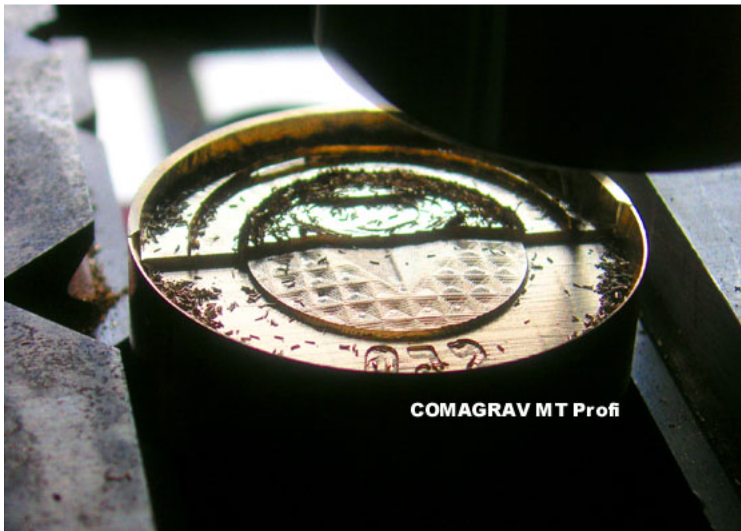
COMAGRAV MT Profi engraving of 3D brass mold
