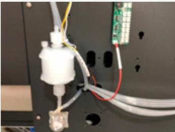
Our filter not only effectively captures large particles, gels and other impurities, but also allows the required pigment particles to pass through and remain in the ink.
