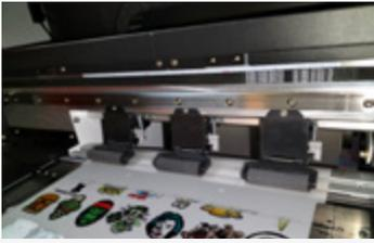
Depending on the printing material, adjust the platen support to adjust the pressure of the pinch roller to ensure smooth film feeding and improve the printing quality. This will increase the friction force during film feeding, making the process more stable and reliable.
