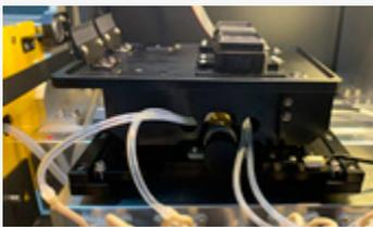
In order to prevent ink from clogging the nozzle, the ink cap will eject some moisturizer every once in a while to keep the nozzle clean and moist. This is the automatic in-line moistening system. It will keep the printer nozzle in the best working state, avoid blocking the nozzles due to evaporation of water in the ink, and prolong the service life of the printhead.
