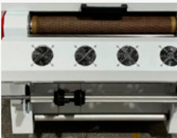
The film feed and take-up with tension system allows you to complete production unattended for a simple and precise workflow from printing to loading and feeding through the roll-to-roll securely wound.
