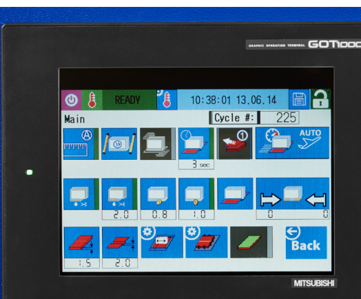
Touch Screen Control Panel
